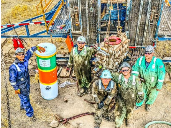
The Plugging Crew sets a Blowout Preventer (BOP) at the A. Lorenzen #15
